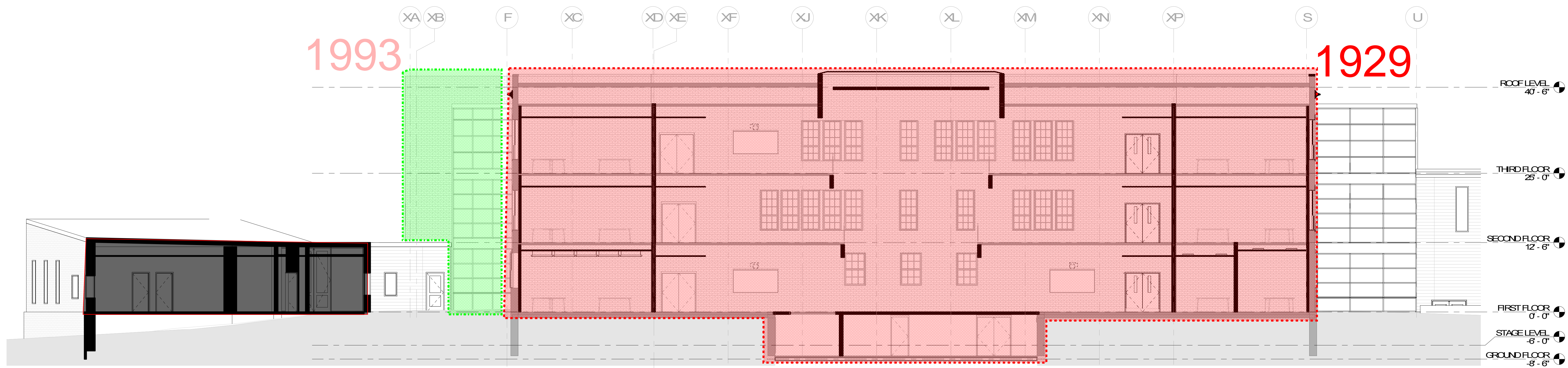
A302 SECTION THROUGH SKYLIGHT ADDED TO CLASSROOM BUILDING 1/8" = 1'-0"
